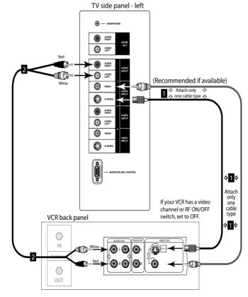
Figure 6. Connecting the VCR Audio/Video.
